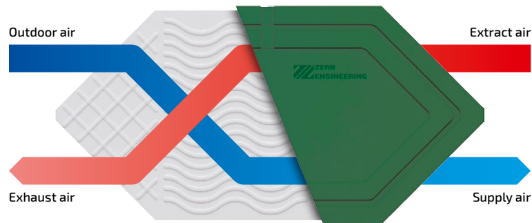
Counter-flow heat exchanger airflow pattern
